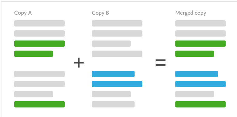
FIG 3.7: In a simple merge, Git finds only the changed lines from two branches and combines them to produce a third, merged snapshot.
